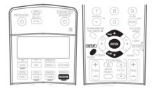
**1** While pressing the RECEIVER button, press SETUP. The remote LCD display shows SETUP.
